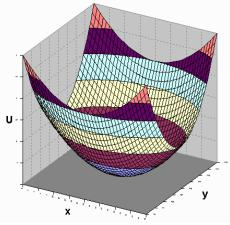
Gradient Gradient is Large Note that far from the "bottom" of the plot, where the gradient is steep, equipotential surfaces are closely spaced. Near the "bottom" of the plot, where the gradient is shallow, equipotential
