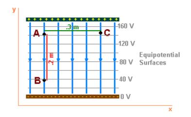
The negative charges have a potential of zero in this example. Note that while A is at 140 V and B is at 40 V, the potential difference between A and B is 100 V, with A being higher than B, just as we said earlier.
