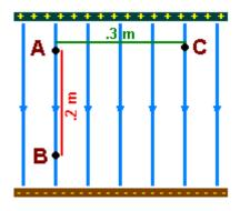
shown. The potential difference between A and B is measured to be 100 V (with A having the higher potential). Well, because A & B fall along a field line, it's not hard to calculate the field strength:
