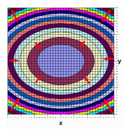
Now we are really determining the field, based on the potential. We can do it almost by looking at it.
