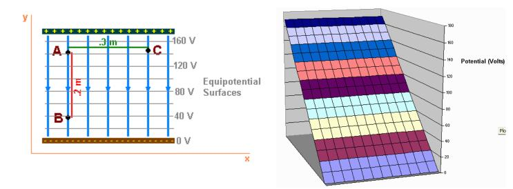
Looking "down" on the surface plot produces an equipotential surfaces plot - also known as a **contour plot**. (Yes, the equipotential surfaces plot is not the same as a surface plot, and a contour plot shows equipotential surfaces. Go figure.)
