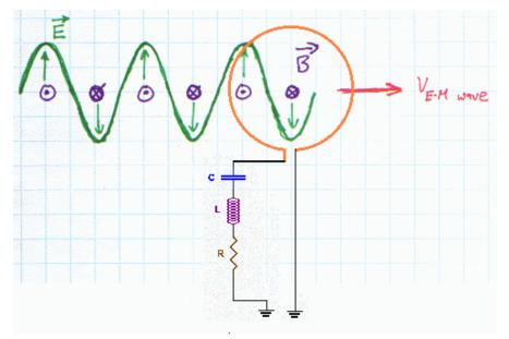
circuit. If the circuit is tuned (by means of a variable capacitor or inductor) so that it resonates with the voltage produced by the EM wave, significant current can be produced in the oscillator circuit, and the signal detected and amplified. This type of antenna, which detects the Bfield component of an EM wave, is called a loop antenna.
