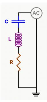
The equation is exactly the same, mathematically speaking, as the equation for the mechanical oscillator. This means all the behavior found in a mechanical oscillator can be found in this system as well. Sinusoidal motions, damped oscillations, resonant behavior - it's all here.
