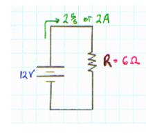
Law. The units of resistance are V/A =  $\Omega$  (Ohms). We can draw a diagram of the above circuit showing the voltage, current, and resistance in a simple form as shown at left.
