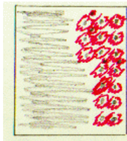
Here the pink indicates violent vibration of molecules in object A, which is hot.
