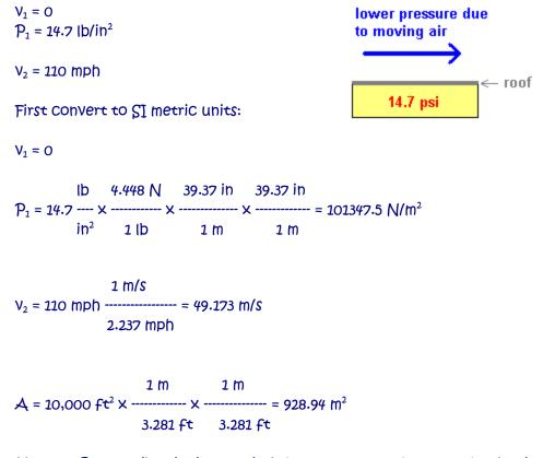
Now use Bernoulli's principle to find the pressure on the roof (the density of air is  $\rho = 1.29 \text{ kg/m}^3$ ):
