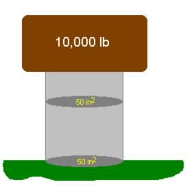
F P = ---А F (d) Work Energy [Joules] P = ----- = ------ = ------A (d) Volume Volume [m<sup>3</sup>] The units work out, too: [J] [Nm] [N] P = ----- = Pascals = Pa [m<sup>3</sup>] [m<sup>3</sup>] [m<sup>2</sup>]
