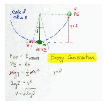
This gives me speed at the bottom of the swing. At that point the forces acting on the swinger are the Tension in the Chains and the swinger's weight. Because the swinger is moving in a Circle, the total force on the swinger must be equal to his mass times his Centripetal acceleration.
