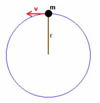
From a vector perspective, the velocity is changing. Therefore the mass is accelerating because  $\mathbf{a} = \Delta \mathbf{v}/t$ . The velocity vector is always being re-directed toward the center of the circle, so the acceleration is centripetal ("center-seeking"). The centripetal acceleration is given by
