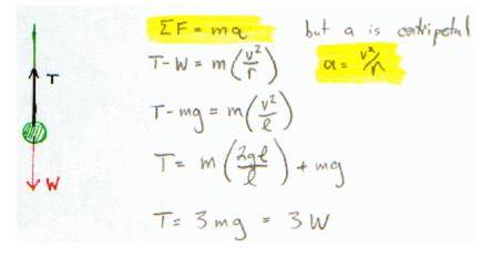
So the Tension in the Chains is three times the swinger's weight.
