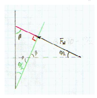
A little high school geometry in action! So  $F_N$  is directed at and angle  $\theta/2$  above the horizontal. The problem is symmetrical so  $F_N$  should be the same on both sides. Now split into components and do the usual vector stuff:
