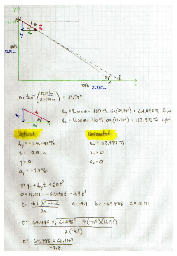
t= .1864 sec (the other solution is negotive) Plug into harizantal info: X= X0 + Vox + + + = 9x+2 X= 0 + 122.872 1/6 (.18645) + ± (0) (.1864) X= 21.039m X= 21 m The arrow hits at 21 m. The target is at 21.3m So the arrow falls any .3 in or 30 our short of the mork.
