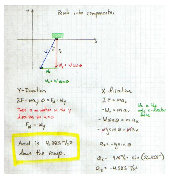
Now rotate the axes so I have the usual x-y Cartesian coordinate system and get to work.
