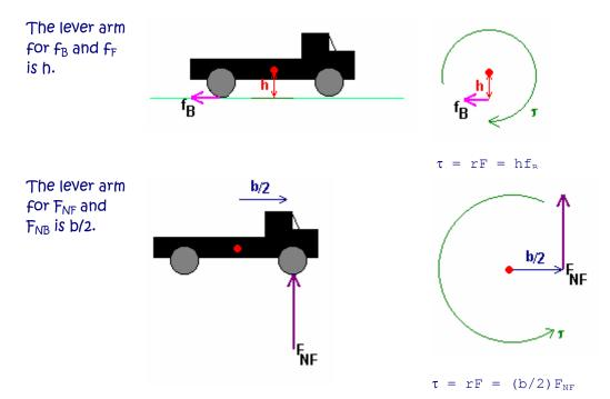
The torque caused by the normal force on the front tire is counter-clockwise. The rest are clockwise. I'll call clockwise positive
