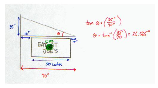
The sign is a rectangle -- the center of mass lies at its geometric center. Then once I know the distances I will move on to dealing with forces and torques. They all must cancel out -- all torques and forces must add up to zero. I'll start with torques first to find the tension.
