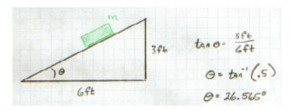
I guess slippery means friction is not significant. So the only forces acting on the Child are gravity (weight) and the normal Contact force between the child and the slide.
