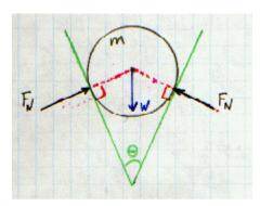
This is another **statics** problem. First I'm going to sketch out the problem. If there is no friction ("slippery sides"), then the only forces that act on the ball are its weight and the normal contact forces between the ball and the walls of the "V"
