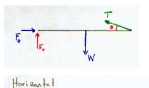
$\Sigma F = ma_x = 0$   $F_{\mu} - T_x = 0$   $F_{\mu} - T_{cos \Theta} = 0$   $F_{\mu} = T \cos \Theta = 22.36 \text{ lb } \cos(26.565^{\circ})$   $F_{\mu} = 20 \text{ lb}$
